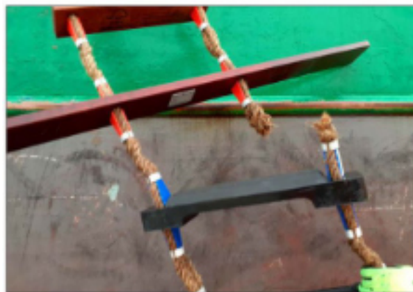
Figure 2: Example of a failed pilot ladder
