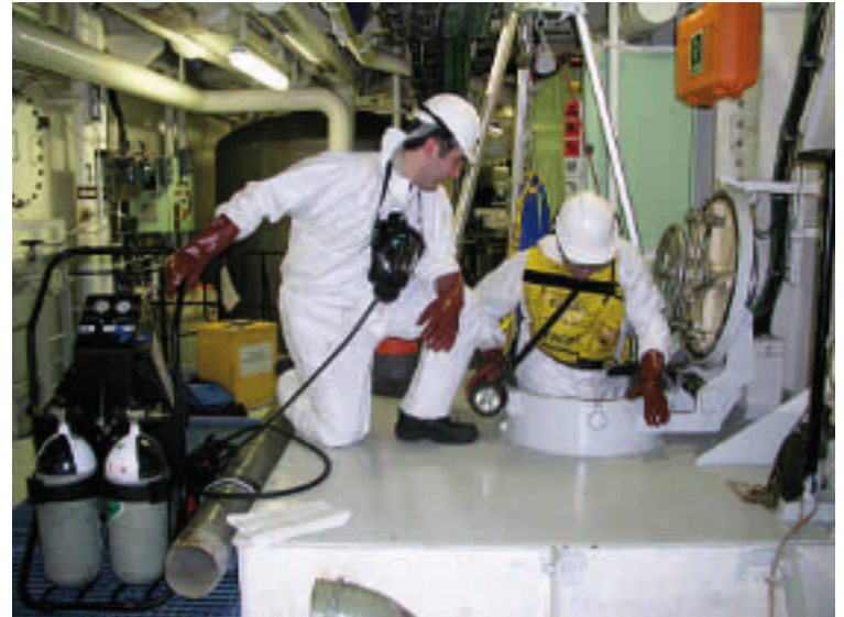
Two men seen working at the entry into an enclosed space.
