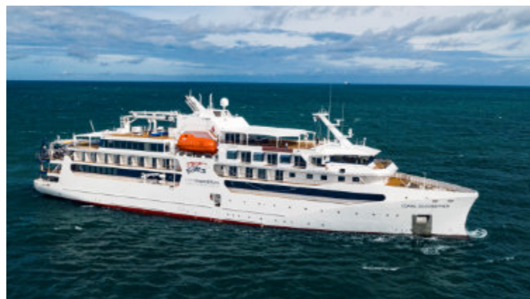
Coral Geographer , Expedition Cruise Vessel, loa 93.7 metres, beam: 17.2 metres. Built to VARD 6 01 design.
